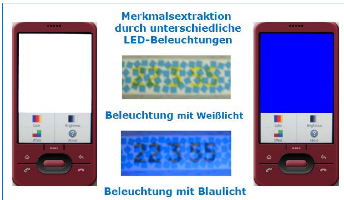
Fig. 04 Object detection with different colored lights [04]
