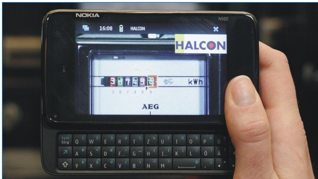
Fig.12a HALCON embedded runs on the Nokia N900 mobile phone [SYMBIAN] [12a]
