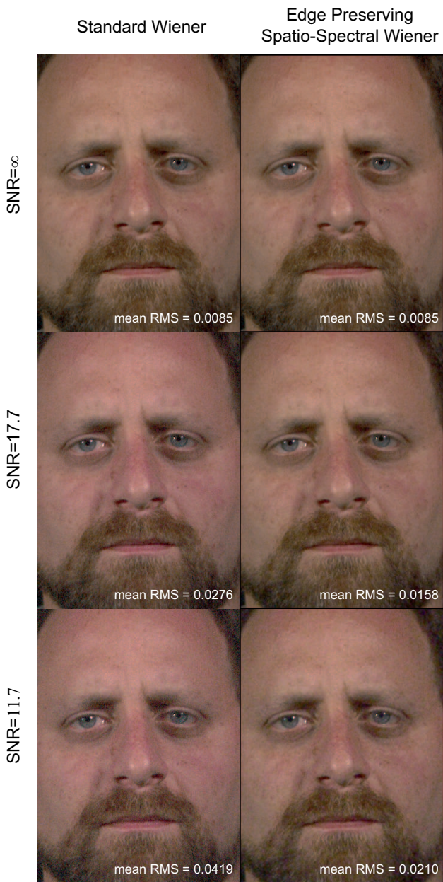
Fig.3: Spectral reconstructions from a six-channel capture of a Lippmann2000 image shown as sRGB renderings. Different noise levels were considered reaching from zero noise to large noise levels.
