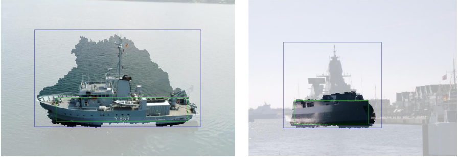
Figure 3: Segmentation results with GraphCut : initial segmentation is given with two rectangles (outside the blue one is background, inside the green one is the object).
